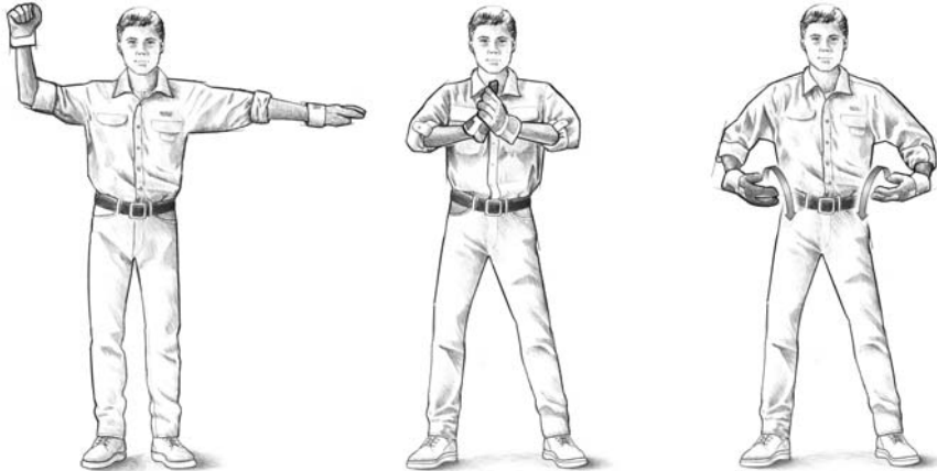
5) Stop the winch Clinch fist, palm to driver, held high enough for driver to see and other arm straight out at shoulder height is the sign to stop the winch.
